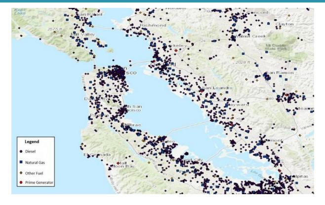
Diesel capacity growing as back-up 6,500 BUGs throughout the San Francisco Bay Area, not counting backyard generators, nearly four gigawatts of electricity, and producing upwards of 259,000 pounds of CO2 a day, and other emissions.
